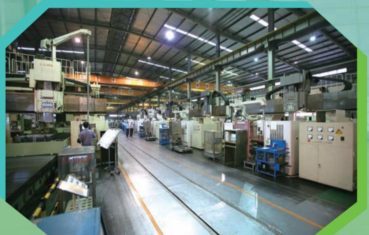
Production line for extra large size mould bases, with over 20 tonnes table loading capacity, to provide services to customers engaged in the manufacturing of auto-parts, and household electrical appliances
