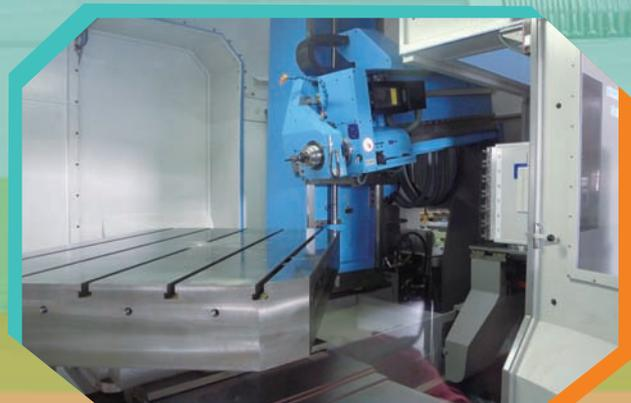
The newly installed 5-axis deep hole-drilling machine is able to produce deep holes on different planes and angles, providing more options in the design of the cooling channels and parts ejecting system
