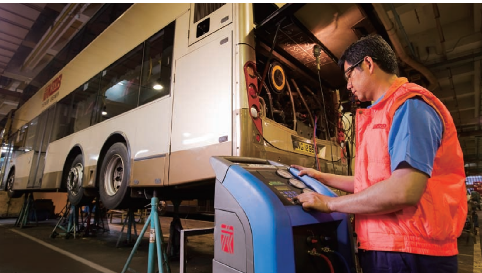
Our refrigerant recycling machine facilitates the maintenance of bus air-conditioning systems in an environment-friendly manner
