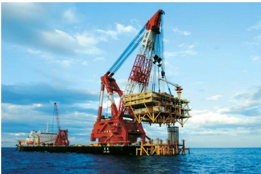
"Lan Jing", the world's largest 7,500-ton full-rotary floating crane, developed by ZPMC, completed its first hoist smoothly as delivered for use
