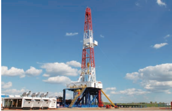
5,000 meter digitally-controlled VFD rig sold to the domestic market
