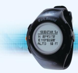
GPS watch that tracks your location and altitude with built-in compass and memory of up to 10 previous trail data with electronic directional map.
