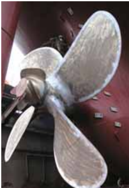
The use of propeller boss cap fins increases the fuel efficiency of our owned ships
