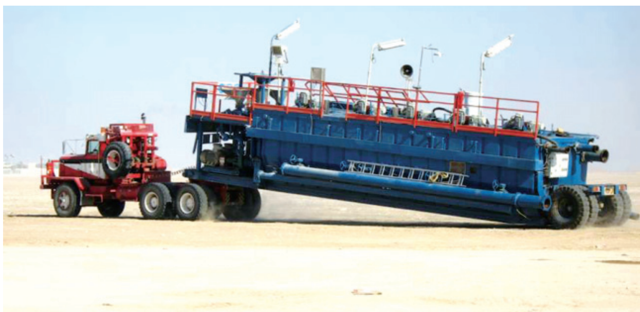
Transportation for mud tanks
