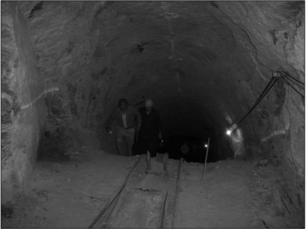
Access/Hoisting Downdip Roadway Into Production Cell Under Development
