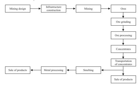
We use different smelting processes to smelt different metals. These primarily include the thermal reduction process and the electrolysis process. The following diagram shows our copper ore smelting process to illustrate our smelting operations:
