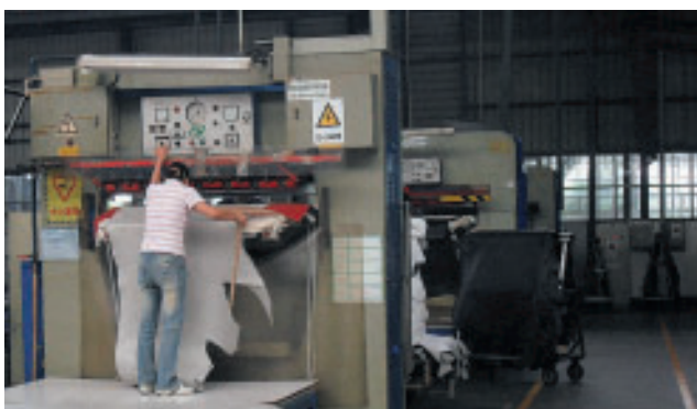
Processing machine with safety features at the Prime Asia Leather Factory to emboss fashionable patterns into the leather for use in the manufacture of shoe uppers. (Huangjiang Dongguan) 東莞黃江的普愛亞細亞皮革廠房備有安全裝置的加工機器，將時尚圖案裝飾在用作製造鞋面的皮革上。
