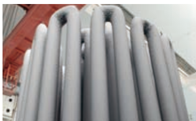
Polysilicon from reactor
