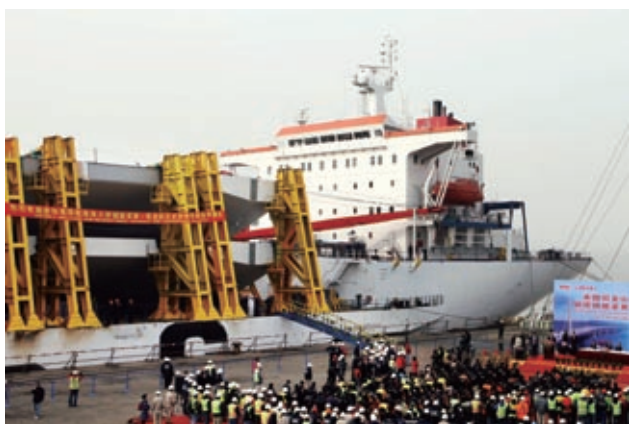
Steel-box girder transport for U.S. New Bay Bridge
