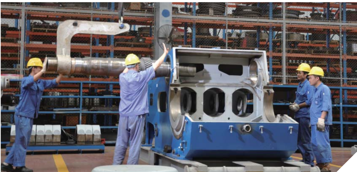
Assemble the mud pump
