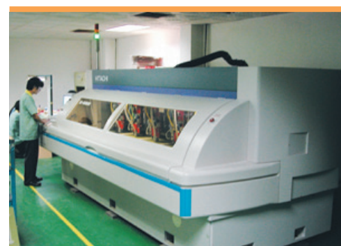
One of the Drilling Machine in Dongguan Plant
