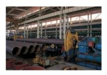
According to customers' requirements, the welding steel pipes are usually beveled at the ends for better joint effect between pipes. The expanded steel pipes are then transferred to the edge trimming machine for process.
