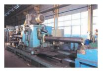
The steel pipes will be tested by ultrasonic testing machines again for invisible defects before they are cut into their designated lengths according to customers' specifications. After cutting, the steel pipes will have plain ends.
