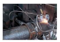
After forming, the skelp edges still remain in the steel pipes. The steel pipes are then fed into a high frequency welder which heats the longitudinal edges of the strips to a very high temperature. The skelp edges are sealed together by welding. The heated edges are then squeezed together to form a fusion weld. After the welding process, the pipes still need to be deburred to remove excess weld beads on both the inner and the outer surfaces of the steel pipe.
