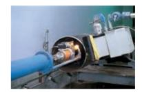
After edge-trimming, the quality control staff will conduct quality tests using ultrasonic and X-ray testers, then they will assess the exterior and interior quality of the steel pipes. The quality inspection results and the mechanical properties of the steel pipes have to meet certain requirements.
