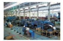
The uncoiled rolls of hot rolled steel coils are cut into strips of predetermined sizes to form steel pipes of specific dimensions before they are fed into the forming machine. An electrically operated shear cuts off the end of each coil and the coils are then welded together to form a continuous strip. The continuous strip is then accumulated at the super accumulating unit to ensure that the forming unit is fed with a continuous strip of steel in the production process.
