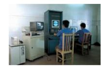
After edge trimming, the steel pipes will be inspected for invisible defects using ultrasonic testing machines and X-ray machines, with the surface polished according to appearance requirements, and conduct various mechanical property tests and examinations.
