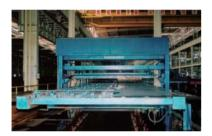
First of all, to ensure that the raw materials meet the technical requirements, we will conduct ultrasonic scan on the steel plates using parallel band or grid scanning mode and will examine both sides of steel plates using a turning device.
