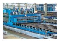
First of all, to ensure that the raw materials meet the technical requirements, we will conduct ultrasonic scan on the steel plates using parallel band or grid scanning mode and will examine both sides of steel plates using a turning device.
