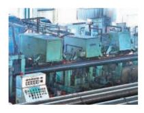
The fusion weld and hot affect zone of the steel pipes are subject to heat treatment, which will increase the mechanical strength and hardness of the steel pipes. The heated pipes will then be air and water cooled.
