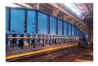
After the ultrasonic test, both longitudinal sides of the steel plates are to be milled according to width specification requirements. Precrimping the sides of steel plates is a necessary process to obtain an ideal arc of steel pipes and in consideration of the inner stress effect after welding.
