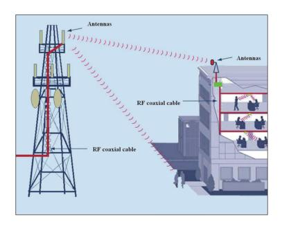
The following diagram illustrates the application of leaky coaxial cables:
