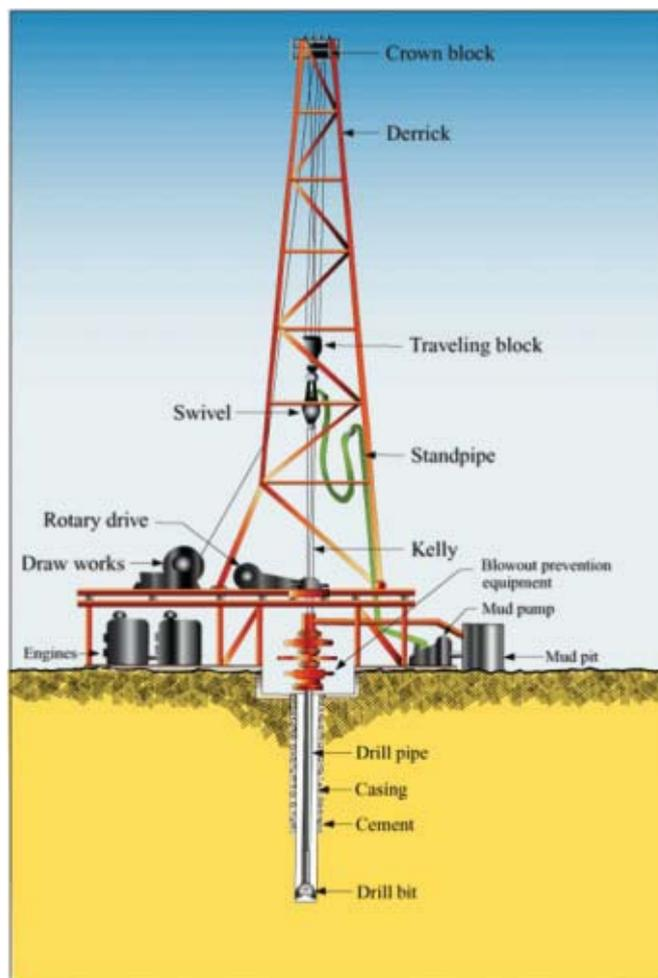
Figure 1: Schematic of an onshore drilling rig
