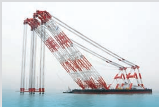
8000t floating crane
