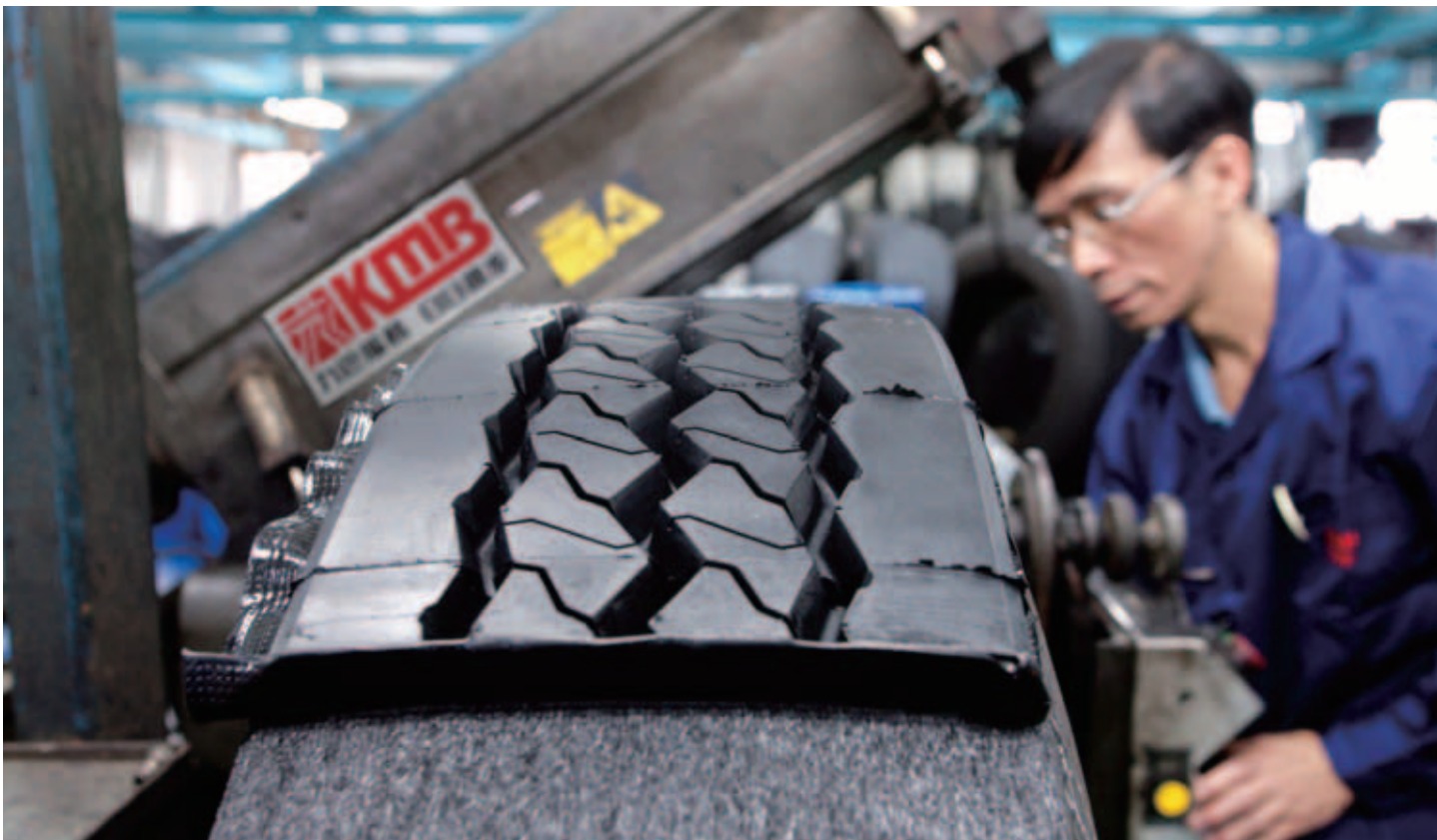
KMB retreads tyres for environmental preservation
