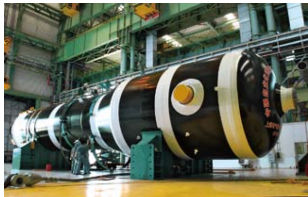
1000MW Class Steam Generator
