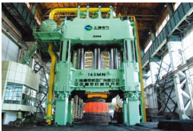
16,500-ton free-forging hydraulic press
