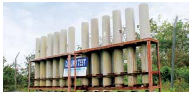
Column testing of waste materials at Martabe.
