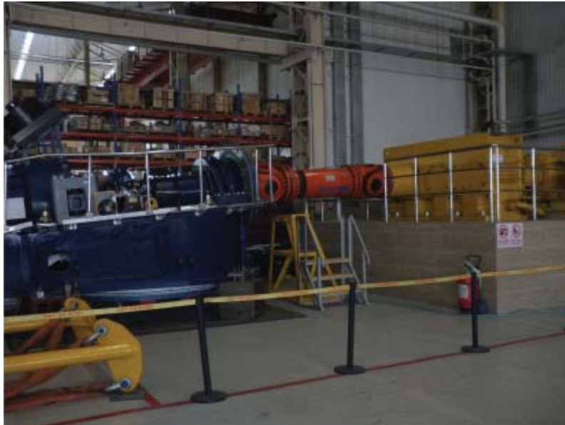
Figure 2.3—Nacelle final test
