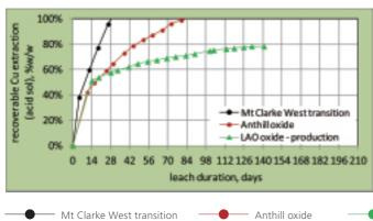
ANTHILL OXIDE, MT CLARKE WEST TRANSITION AND CURRENT PRODUCTION ORE ACID CONSUMPTION CURVES (BASED-CASE TEST COLUMNS ONLY)
