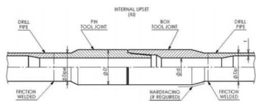
**Drill Pipe with Weld-On Tool Joint Assembly**
