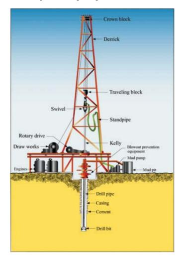
Figure 1: Schematic of an onshore drilling rig
