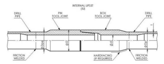
Figure 2: Drill Pipe with Weld-On Tool Joint Assembly<sup>7</sup>
