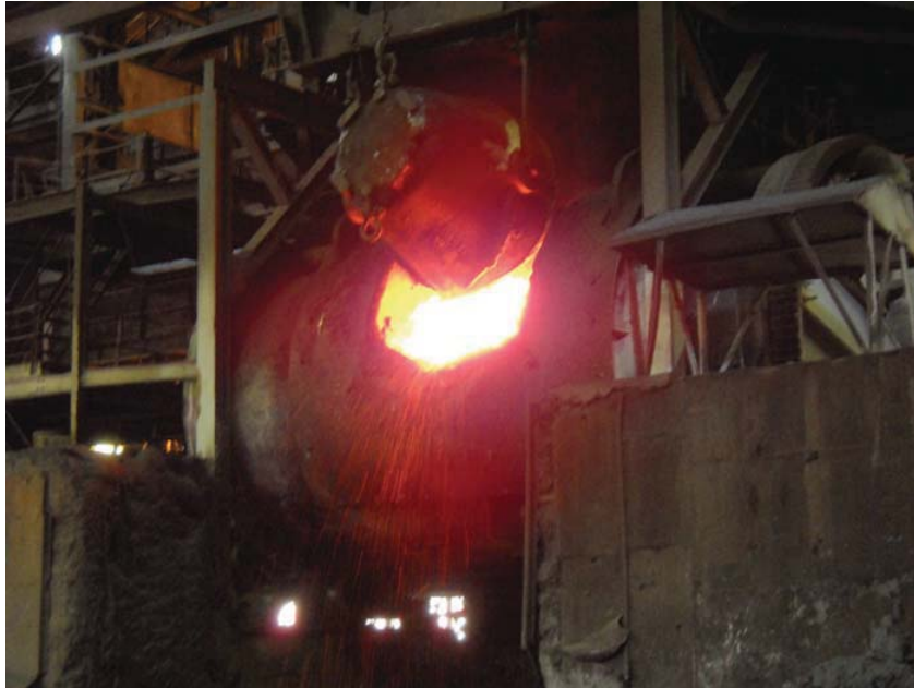
Figure 55: Molten Metal "Matte" being poured into the Converter
