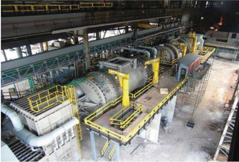
Figure 57: New Anode Furnaces each of 400T Capacity
