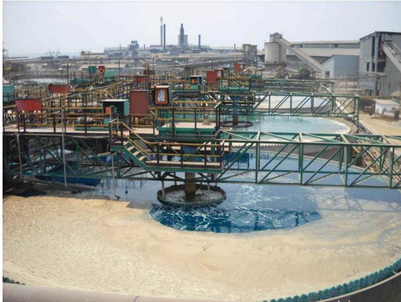
Figure 43: The Oxide Plant CCD Circuit
