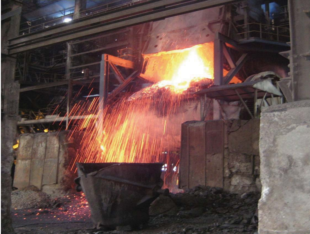
Figure 56: Old Converter in Operation
