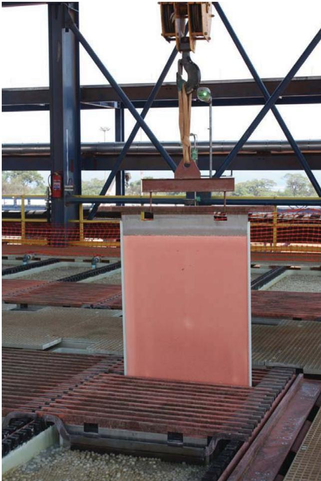
Figure 61: Copper Cathode from the Heap Leach Operation in September 2010
