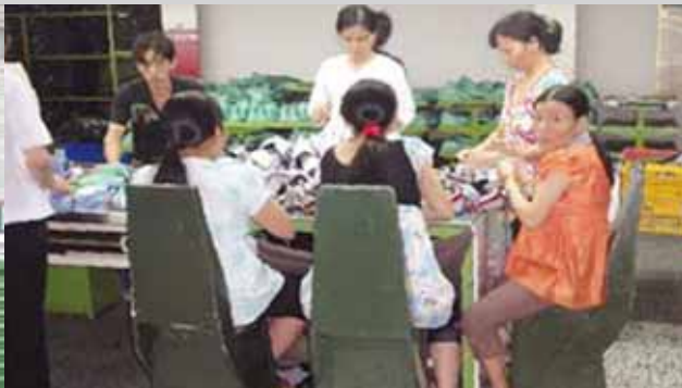
4. The factory designed a chair anatomically suited to pregnant staff 工廠設計一張結構適合懷孕員工的座椅
