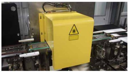
Solar WIS - resistivity and P/N type measurement
