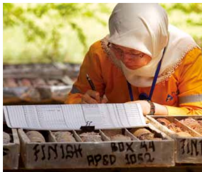
A geologist records the geological log of a Tor Uluala drill hole prior to interpretation and 3D computer modeling.
