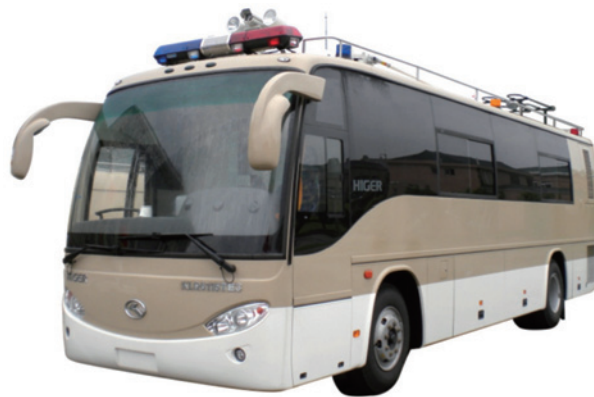
Large scale VSAT high speed dynamic satellite system communication vehicle
