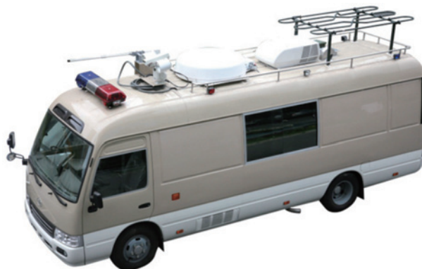
Medium scale VSAT high speed dynamic satellite system communication vehicle
