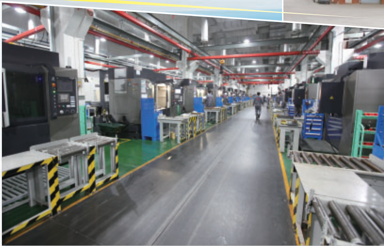
▲ 中小型精密模架生產線。 Production line for small and medium size high precision mould bases.
