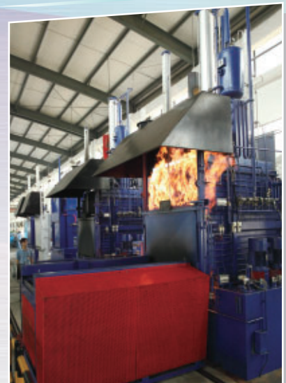
▶ 多功能熱處理爐用於大批量生產模架零配件。 Multi-purpose heat treatment furnaces for mass production of mould base components.
