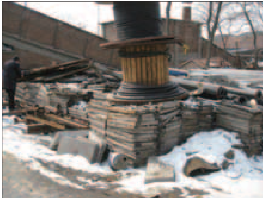
Figure 7-10: Current storage facilities and condition of drill core for the project
