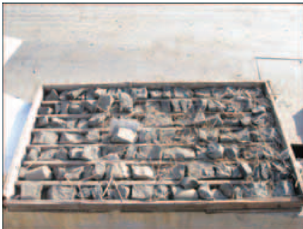
Figure 8-13: Drill core from ZK204-1 (87.20-89.50 m)
