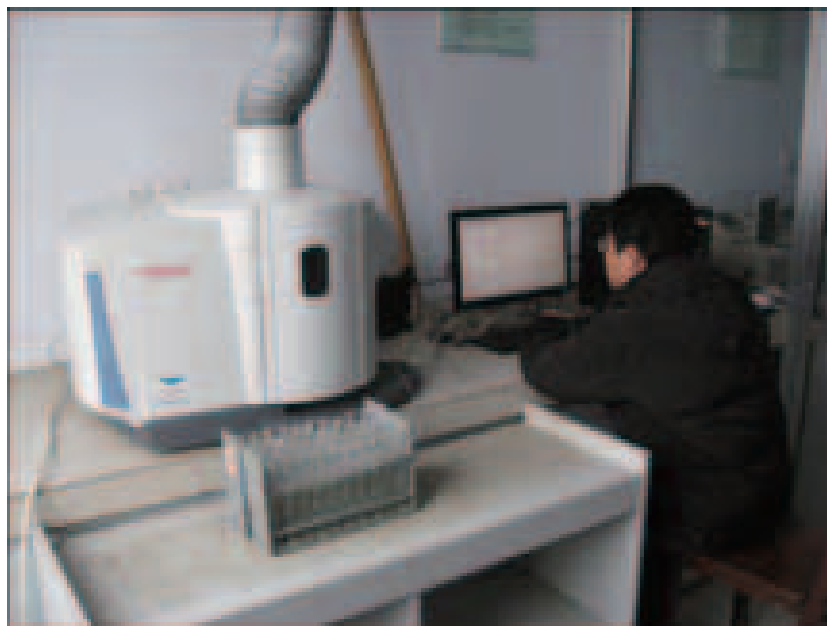
Figure 8-9: Technician operating ICP-OES machine at the primary Rizhao laboratory
