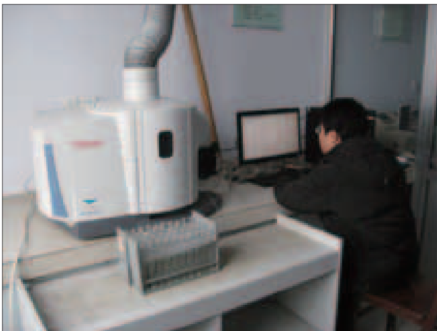
Figure 7-9: Technician operating ICP-OES machine at the primary Rizhao laboratory
