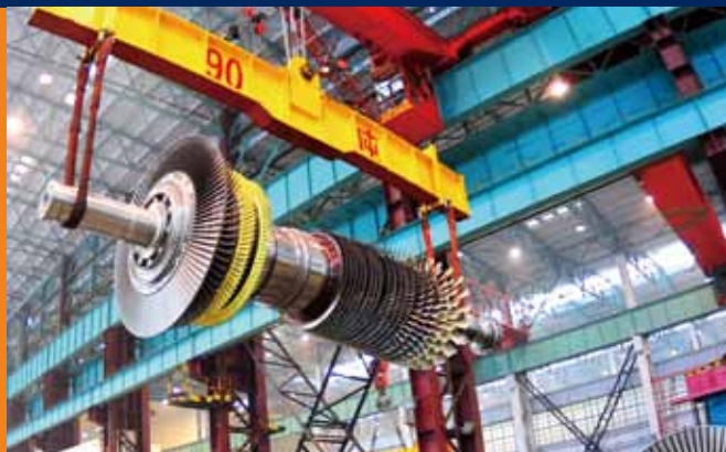
▲ E-model heavy-duty gas turbine rotor
