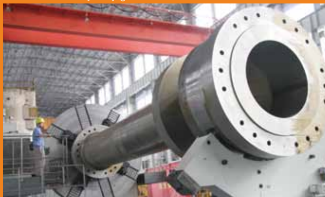
▲ Generator shaft for the Gerry Project in Brazil
