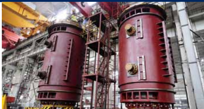
Two 600MW gas turbine generator stators are laminating
