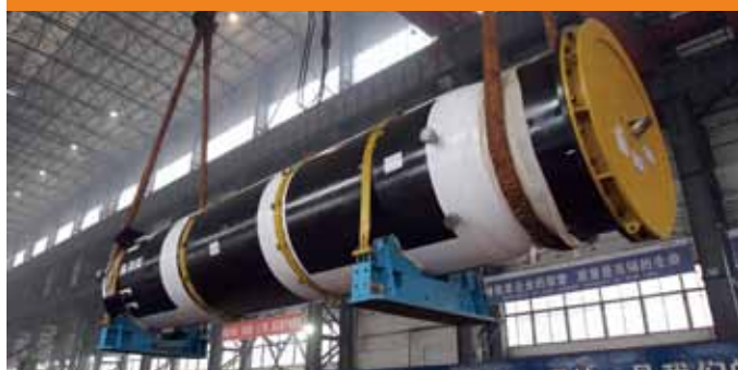
Ready for shipping of 1# generating unit pressurizer at Ningde
