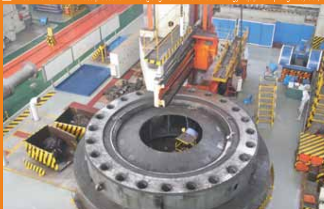
▲ A hydroturbine headcover is being processed on a vertical lathe in Jinping Power Station
