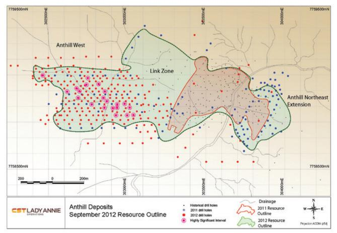
Figure 8: Anthill deposits, showing drill holes and resources
