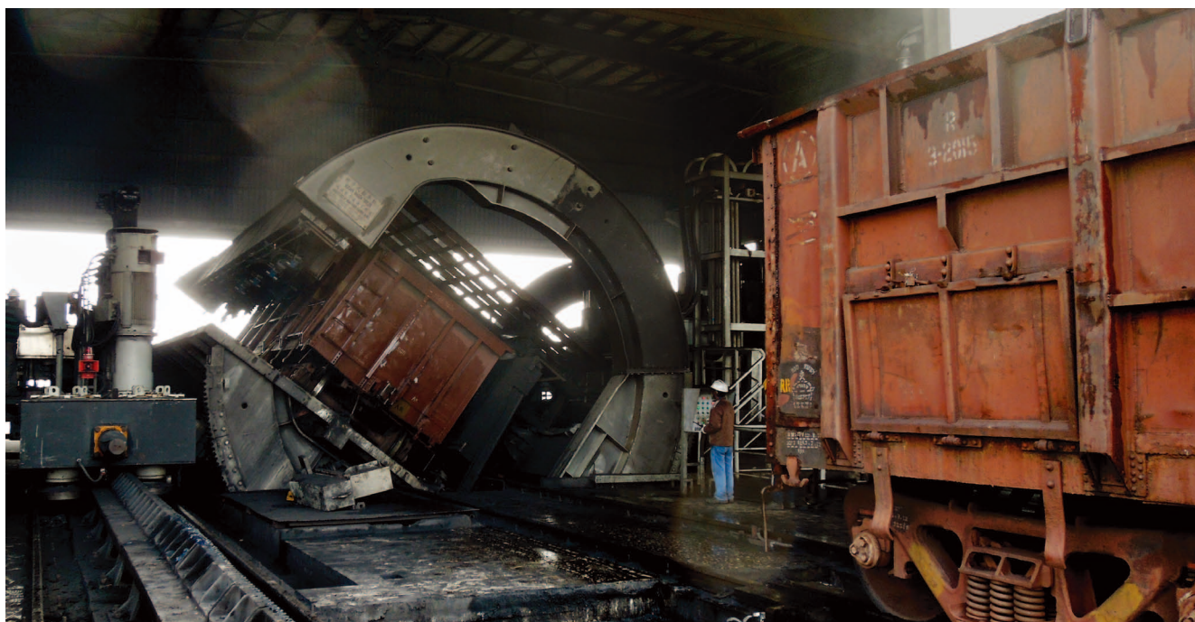
A coal tippler at Jhajjar – we need to unload each train of around 60 wagons within five hours
