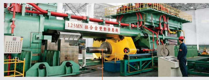
The Group is equipped with a range of advanced large-scale extrusion production lines, with core equipment imported mainly from Europe. These facilities enable the Company to produce large-section, high quality, high value-added aluminium extrusion products on a large scale.
