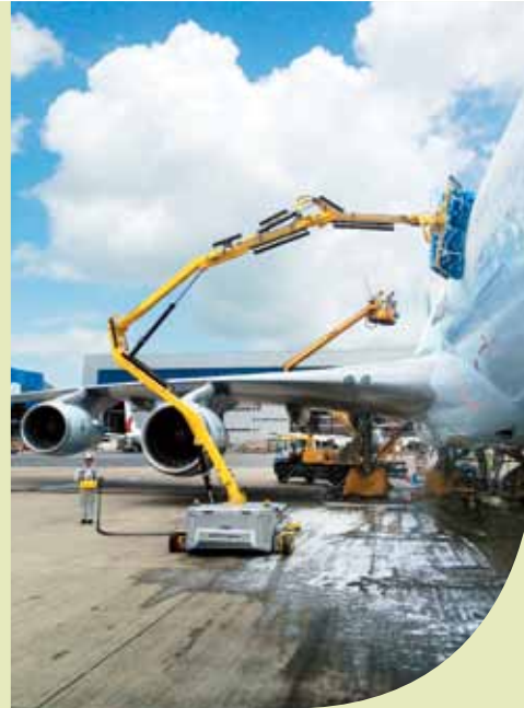
Introduction of a new automated aircraft cleaning system which reduces water consumption and raises occupational safety
