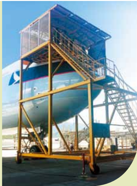
A working platform with solar powered navigation system tailor-made for the repair of aircraft windshield
