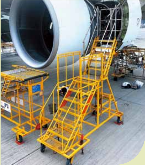
New servicing steps used in line maintenance enabling staff to adjust the height easily
