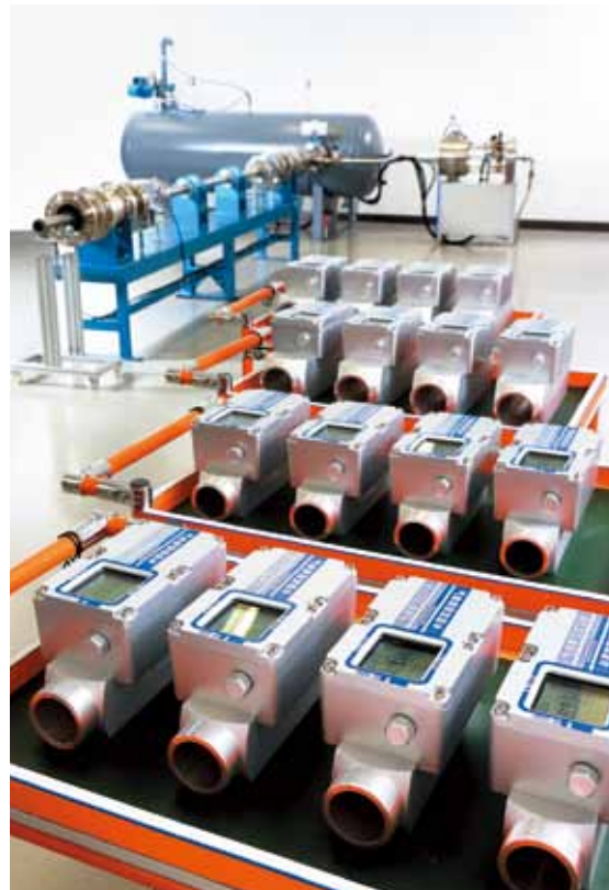
M-Tech's new generation of gas meter uses Micro-Electro-Mechanical Systems technology to measure mass flow and is now in production at the manufacturing plant in Longgang, Guangdong province.
