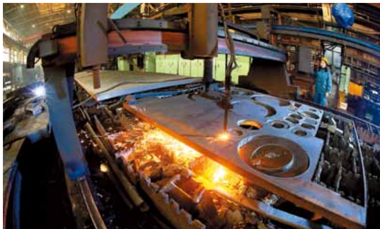
Natural gas torches are used to cut machine tools by a large-scale manufacturer in Jinan.
