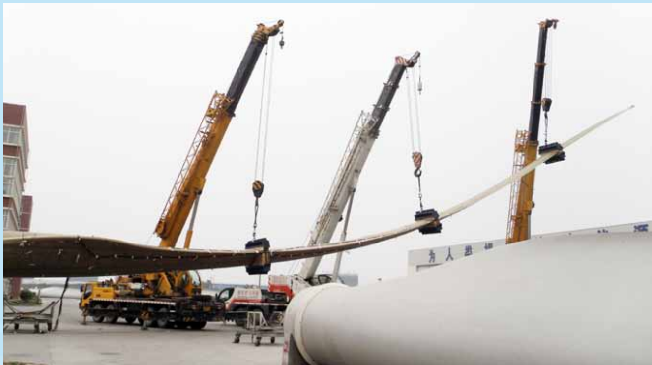
Tests for the first 1.5MW-47m blade was passed 首支1.5MW-47m葉片順利通過試驗測試
