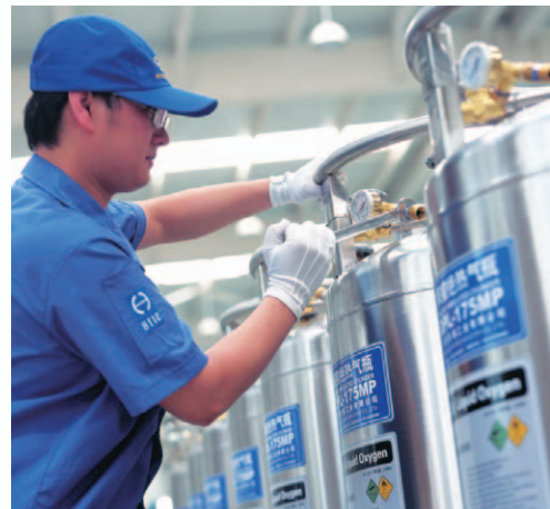
Inspection and repair of welded insulated cylinder
