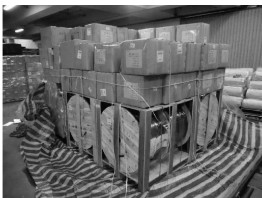
The photograph above shows consolidation of light weight/small volume cargos loaded on top of heavy weight/large volume cargos.
