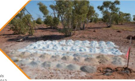
Figure 1: 1m Samples from 70m Rotary Air Blast (RAB) drill hole ready for spear sampling into 4m composites for assay – Lindsay's Lament Prospect
