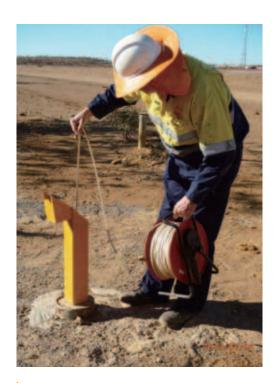
> Figure 3: Checking Water Levels in Bore
