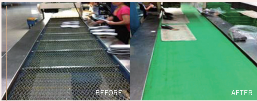
Replacing iron conveyors with rubber belt conveyors
