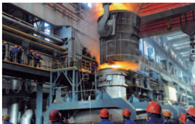
VC large steel ingot vacuum casting equipment with de-dusters installed by CITIC Heavy Industries
