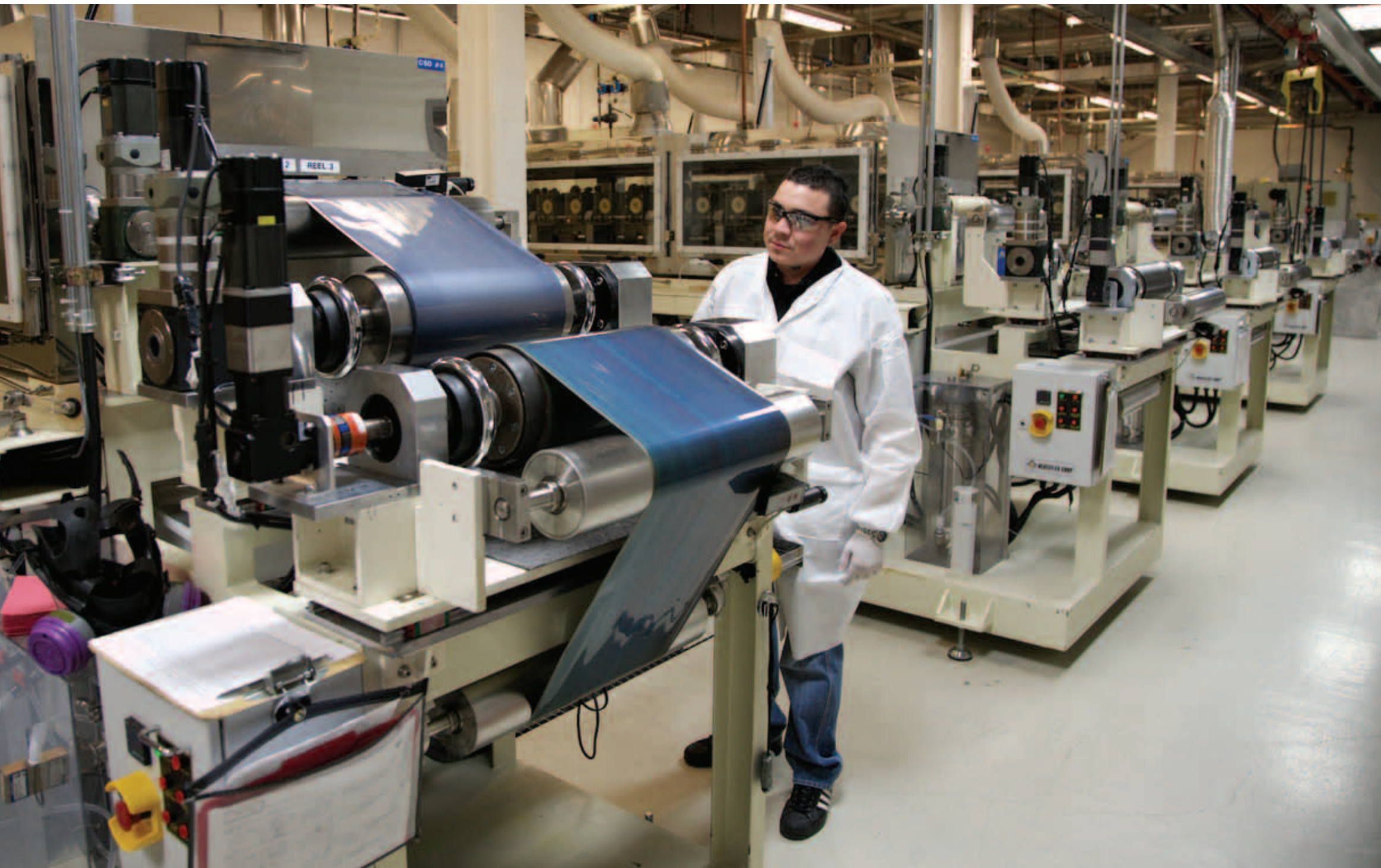
CIGS flexible thin film production line 銅銦鎵碲柔性薄膜生產線
