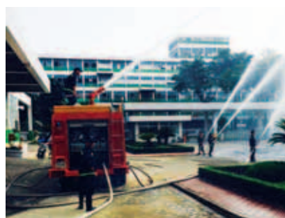
Water pressure test carried out by the fire fighting vehicles and fire hydrants of a factory 廠區消防車與消防柱水壓測試
