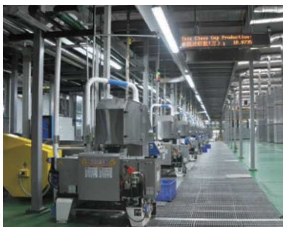
Stretching equipment of Guangzhou Company's two-piece can production line
